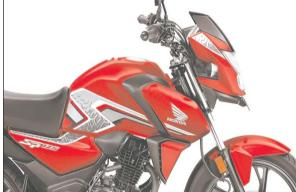
785 mm in width, and 1103 mm in height, providing a well-balanced and compact profile. With a wheelbase of 1285 mm and a ground clearance of 160 mm, the SP125 ensures stability and ease of manoeuvrability on diverse road conditions. The seat height of 790 mm strikes a balance between comfort and accessibility for riders of varying heights, while the
